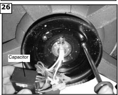
Tighten the three screws securely holding the plate for the switch housing. Remove the double sided tape from capacitor and stick capacitor to plate.
